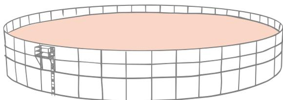
**Liquid storage systems** commonly include round or rectangular steel, concrete or earthen storages with either a clay or synthetic liner. Other options include flush barns or above-ground concrete silos, though the latter is increasingly rare. Liquid manure storage structures should be sized appropriately to contain wastewater as well as rain and snow. Yard runoff should be diverted away from manure storage.
